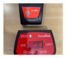
Push 'Print' on the Brake Check. \*Do not move the Brake Check before printing is complete\*
